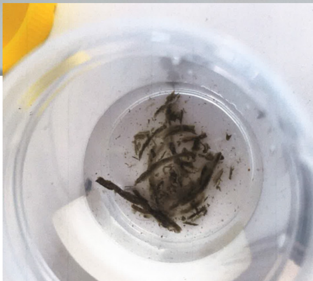
Specimen jars showing the cloudy water, sludge and debris, which was coming out of the taps at the community.
